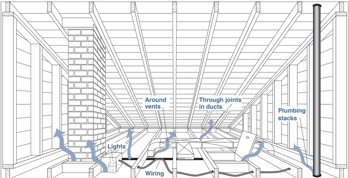
Figure 1-2- Common air leakage pathways through attic floor
