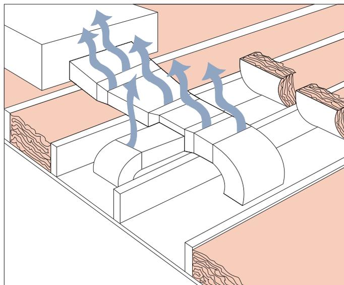
Figure 1-11 - Duct Leakage
