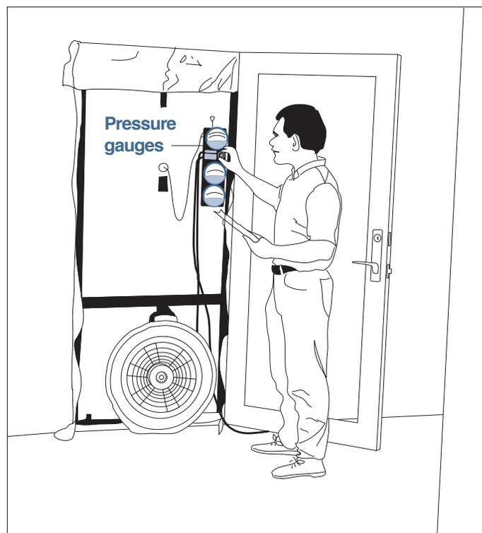
Figure 1-14 - Blower door for testing air leakage.
